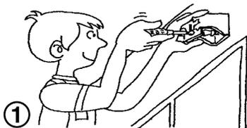
Firmly screw **3630** brackets to wall or ceiling. The two outside brackets should be located 12.5cm (5") in from the ends of track to provide stability. Remaining brackets should be equally spaced along track (approx. every 60cm/2').
