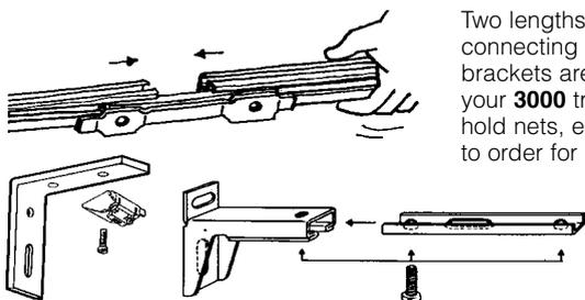
Two lengths of **3000** can be joined with a **3620** connecting bridge. Fixed or adjustable extension brackets are also available to enable you to use your **3000** track with a second Silent Gliss track to hold nets, etc. Ask your dealer. **3000** can be bent to order for bay windows, etc. from your stockist.
