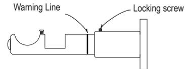
6. Fix the remaining brackets around the window in the desired positions, with a bracket at each pole joint position. On sections without joints you should also ensure that the brackets are no further than 2 metres apart.
