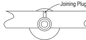
5. When used correctly this bracket is extremely strong but when fitting you should always ensure that the warning line which is engraved around the barrel is **NOT** showing.
