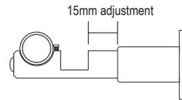
4. The joining plug that fixes the sections together should ideally be positioned over the centre of each bracket.
