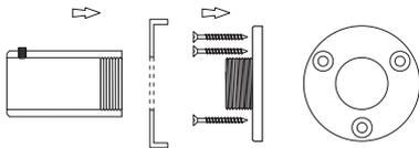
3. The pole is placed into the small semi-circular recess in the bracket and secured with the small screw at the back. A small amount of adjustment is present in the bracket, as below.
